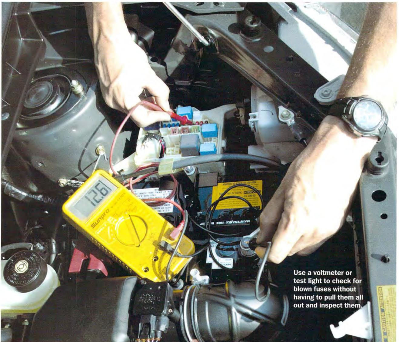
Use a voltmeter or test light to check for blown fuses without having to pull them all out and inspect them.
