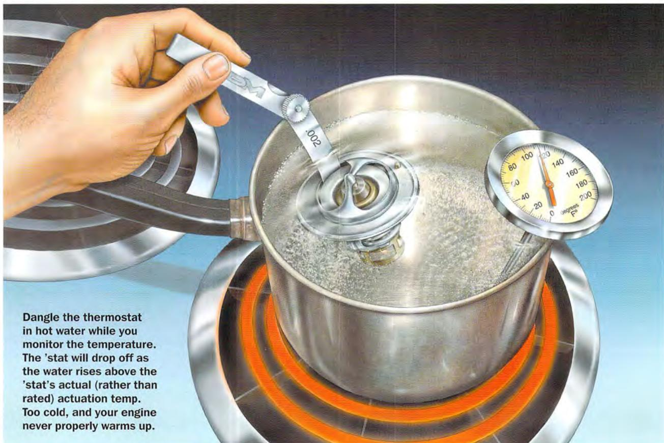
Dangle the thermostat in hot water while you monitor the temperature. The 'stat will drop off as the water rises above the 'stat's actual (rather than rated) actuation temp. Too cold, and your engine never properly warms up.
