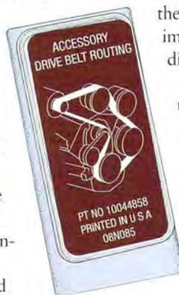
**(Fig. 5)** Vehicles with serpentine belts have a belt routing diagram under the hood somewhere. Read and obey.
