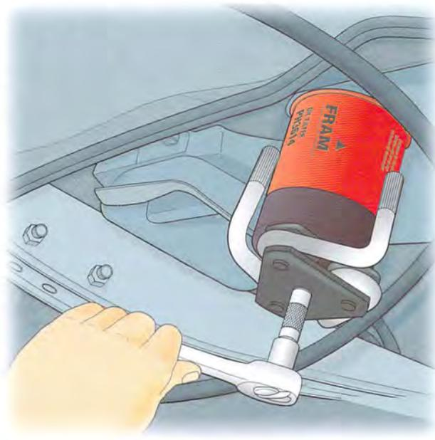
**A spider-style wrench may be more suitable for filters that are not easily accessible.**
