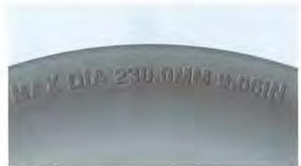
(Fig. 2) Brake drums will be marked clearly as to how far they can be machined safely to remove out of round.
