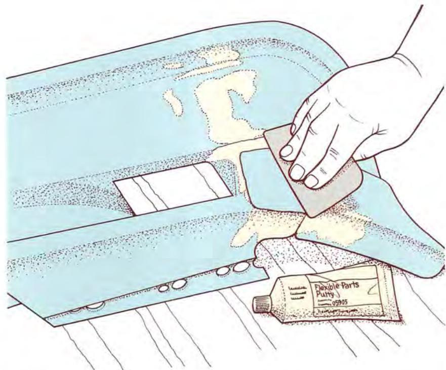
(Fig. 6) The spot repair putty can then be used to fill in scratches, pinholes and small imperfections. It's easier to sand than the repair epoxy.
