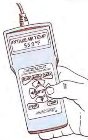
lated load" value and sometimes switch position signals (Fig. 2). OBD II also includes a "capture" mode, in which you can use the scan tool to take a "snapshot" of what the sensors were reading at the exact instant a driveability hiccup occurred (Fig. 3).
