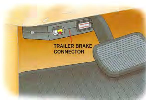
This controller allows the use of electric trailer brakes. Many vehicles are prewired to accept it.
