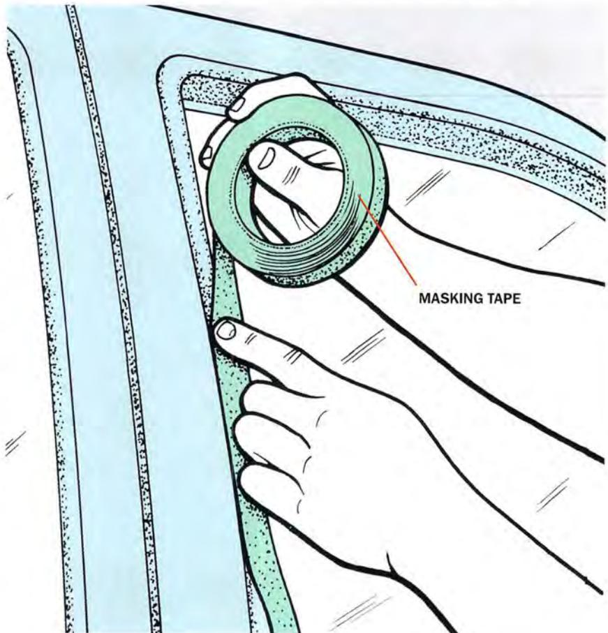
(Fig. 6) Use fresh masking tape to carefully mask all the body trim on the entire car.
