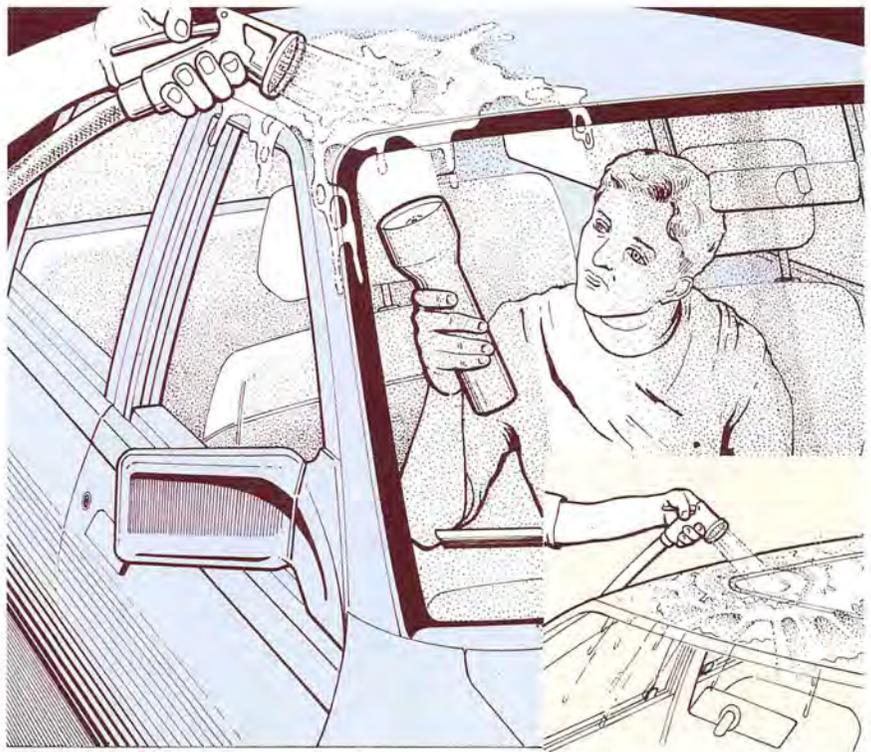
(Fig. 4) Use a helper and a garden hose to follow water leaks back to their source. You may need to remove some trim to find the spot.
