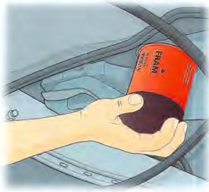
This filter has a rubberized area to provide for tightening by hand.
