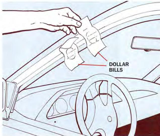
(Fig. 1) A gasket loose enough to let a dollar slide easily might leak air at speed. Tug firmly, but don't tear the bill.
