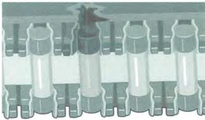
**This glass fuse fuse-box housing melted after a loose clamp overheated.**
