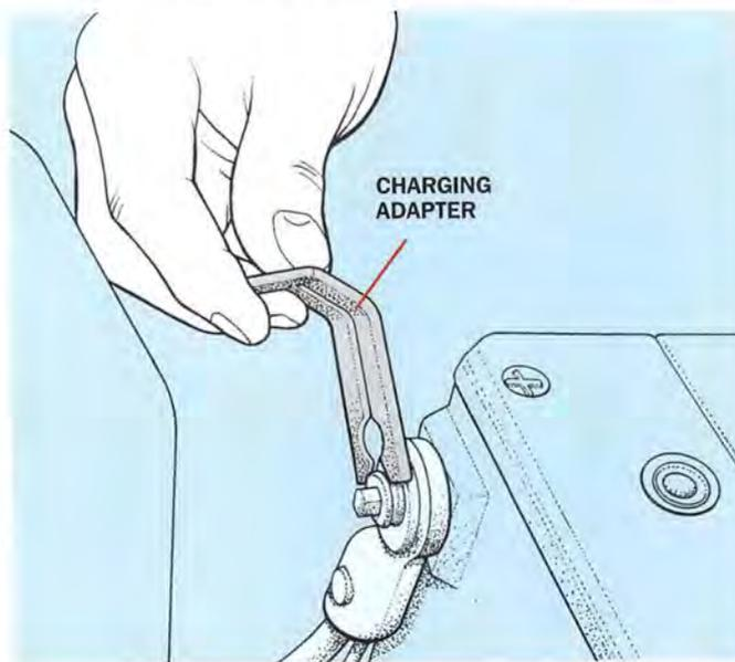
(Fig. 2) It may be necessary to use a battery-charging adapter to let the jumper cables get a good bite on side-terminal batteries.
