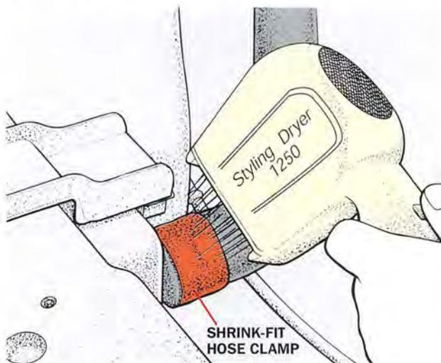
(Fig. 2) Shrink-fit hose clamps will continue to shrink as engine warms up, ensuring a tight seal.
