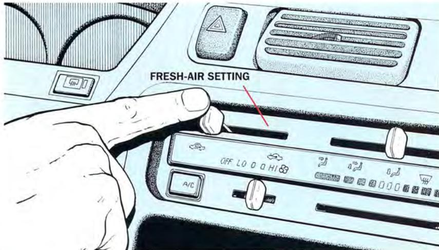
(Fig 1) The simplest cure for odor is to run the air conditioning in fresh-air mode to lower humidity in the evaporator plenum.
