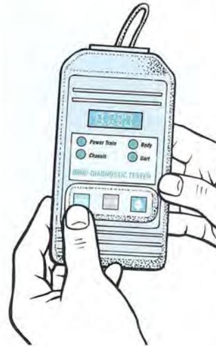
(Fig. 4) Simple code readers/resets like this one do not give you sensor data.
