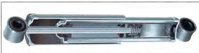
Single- and double-tube shocks are used on either the front or rear end of most vehicles. Struts are simply a shock that includes the spring perch and a bearing that replaces the upper ball joint.
