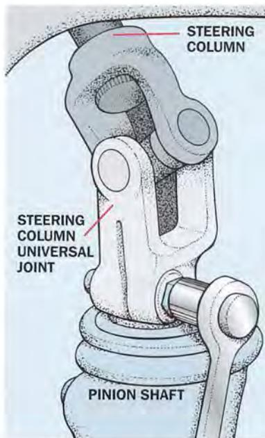
(Fig. 1) Disconnect the rack's pinion shaft from the steering column.
