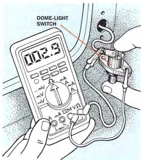
**(Fig. 4)** Check the dome-light switch for intermittent or abnormal resistance with an ohmmeter.
